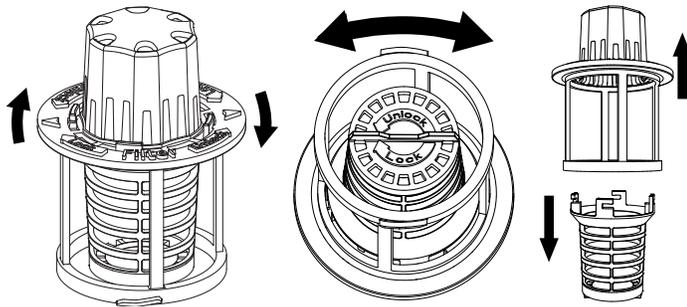
Once cleaned, replace Filter Basket back into the Ultra-Fine Filter assembly and twist it clockwise to lock into place.
